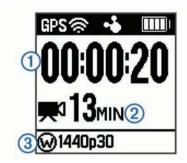
The screen displays the elapsed recording time ①, available recording time ②, and video mode ③.
