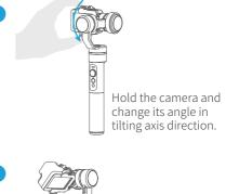
Keep this position for half second, the current angle will be locked manually.
