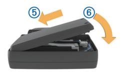
**8** Close the battery cover **6** and tighten the screws. **NOTE:** Do not over-tighten the screws.
